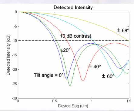
With 0.8 µm deformation we see 10 dB contrast up for a 110° angular aperture
